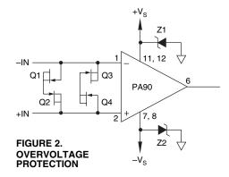
Conditions which can cause open circuits or polarity reversals on either power supply rail should be avoided or protected against. Reversals or opens on the negative supply rail is known to induce input stage failure. Unidirectional transzorbs prevent this, and it is desirable that they be both electrically and physically as close to the amplifier as possible.
