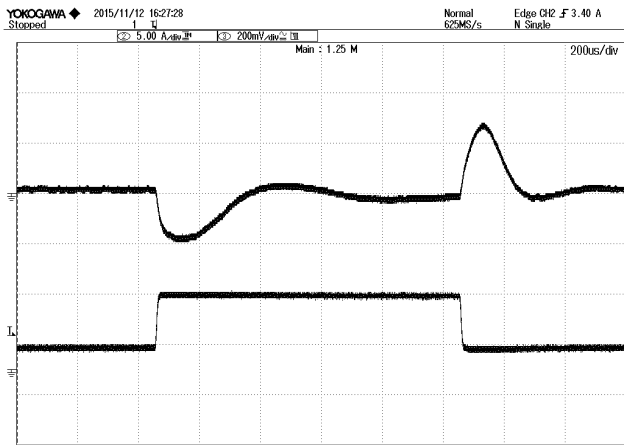
Figure 4: Dynamic response to load step 25%~75%with 0.1A/\mu S slew rate at 220Vac TOP:VOUT, 200mV/div, BOTTOM:Iout, 5A/div, 200uS/div
