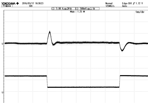
Figure 4: Dynamic response to load step 25%~75% with 0.1A/ \mu S slew rate at 110/220Vac TOP:Vout,500mV/div, BOTTOM:Iout,5A/div, 1mS/div
