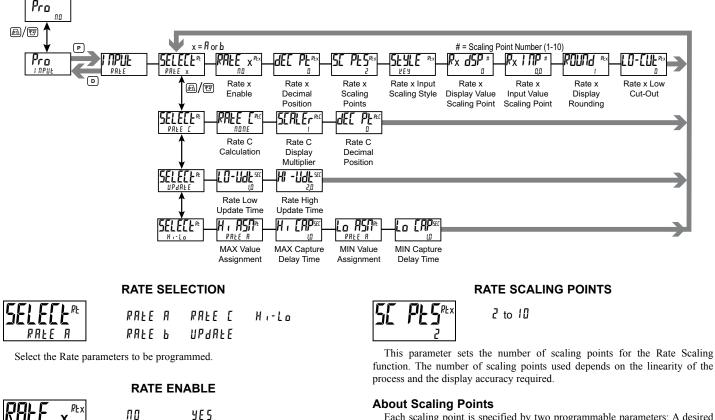
Each scaling point is specified by two programmable parameters: A desired Rate Display Value (Px d5P) and a corresponding Rate Input Value (Px 1). Scaling points are entered sequentially in ascending order of Rate Input value. Each scaling point defines the upper endpoint of a linear segment, with the lower endpoint being the previous scaling point.
