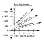
current change. The input summing resistor values are weighted in a binary progression, so they can be switched in combinations to give 32 discrete steps of span. The fine adjust control brackets these coarse steps and can be adjusted to the exact span needed.
