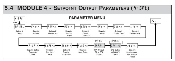
Some Setpoint parameters will not appear depending on the Setpoint Assignment and Setpoint Output Action selected. The Setpoint Parameter Availability chart below illustrates this.
