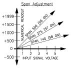
The approximate span contributed by each switch is shown on the rear label. The values shown are "units per volt." For example, if S6 only is turned "ON," the numerical readout will change approximately 550 units for a signal voltage change of 1 volt. If S7 were also turned "ON," the numerical readout would change approximately 825 units for a signal voltage change of 1 volt. The span adjust pot has a continuous span range of approximately 0- 45.
