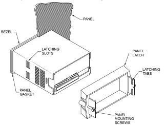
While holding the unit in place, push the panel latch over the rear of the unit so that the tabs of the panel latch engage in the slots on the case. The panel latch should be engaged in the farthest forward slot possible. To achieve a proper seal, tighten the latch screws evenly until the unit is snug in the panel (Torque to approximately 7 in-lbs [79N-cm]). Do not over-tighten the screws.
