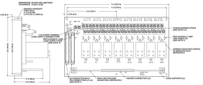
NOTES: 1) CONNECTOR IS CIRCUIT ASSEMBLY CA-50H-2B-SR OR EQUIVALENT. CONNECTORS ARE WIRED IN PARALLEL.
