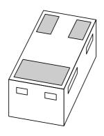
PBSS2515M 15 V, 0.5 A NPN low V<sub>CEsat</sub> (BISS) transistor
