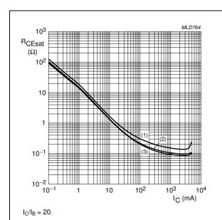
Fig.8 Collector-emitter equivalent on-resistance as a function of collector current; typical values.
