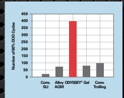
Long Cycle Life ODYSSEY<sup>®</sup> Extreme Series<sup>™</sup> batteries routinely deliver up to 400 deep cycle (80%) discharges.
