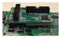
4. Check the screw position of CPU board and PCA-COM232 / PCA-COM485, use threaded spacer and screw to fix.
