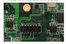
2. Find out the LPC1 connector on PCA-COM232 / PCA-COM485.
