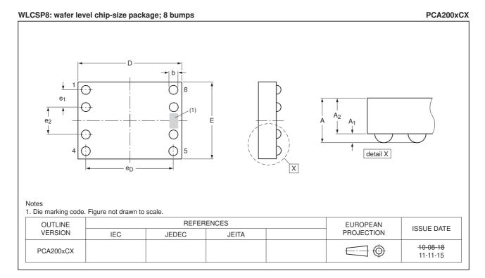
Fig 11. Bare die outline PCA2002CX (WLCSP8) (for dimensions see Table 13, for pin location see Table 14)
