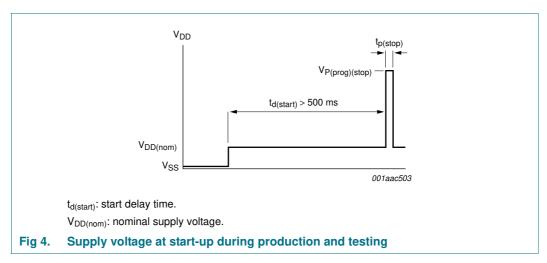
For a watch it is essential that the timing calibration can be made after the watch is fully assembled. In this situation, the supply pins are often the only terminals which are still accessible.
