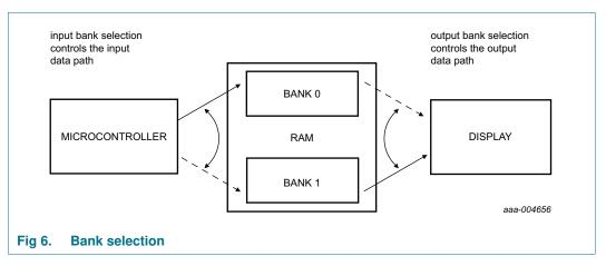
In the static drive mode, the bank-select command may request the contents of row 2 to be selected for display instead of the contents of row 0. In the 1:2 multiplex mode, the contents of rows 2 and 3 may be selected instead of rows 0 and 1. This gives the provision for preparing display information in an alternative bank and to be able to switch to it once it is assembled.
