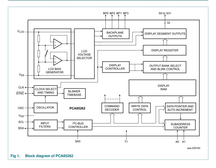
Automotive 32 x 4 LCD driver for low multiplex rates
