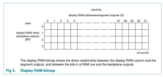
When display data is transmitted to the PCA85262, the display bytes received are stored in the display RAM in accordance with the selected LCD drive mode. The data is stored as it arrives and depending on the current multiplex drive mode the bits are stored singularly, in pairs, triples or quadruples. To illustrate the filling order, an example of a 7-segment numeric display showing all drive modes is given in Figure 4; the RAM filling organization depicted applies equally to other LCD types.
