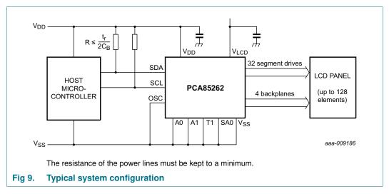
The host microcontroller maintains the 2-line I<sup>2</sup>C-bus communication channel with the PCA85262. The internal oscillator is enabled by connecting pin OSC to pin V<sub>SS</sub>. The appropriate biasing voltages for the multiplexed LCD waveforms are generated internally. The only other connections required to complete the system are the power supplies (V<sub>DD</sub>, V<sub>SS</sub>, and V<sub>LCD</sub>) and the LCD panel chosen for the application.
