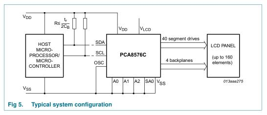
The host microprocessor or microcontroller maintains the 2-line I<sup>2</sup>C-bus communication channel with the PCA8576C.
