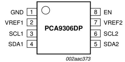
**Fig 3. Pin configuration for TSSOP8 (DP) (MSOP8)**
