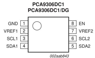
**Fig 5. Pin configuration for VSSOP8 (DC1; DC1/DG)**
