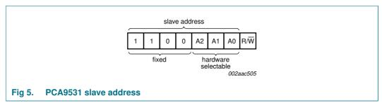
The last bit of the address byte defines the operation to be performed. When set to logic 1 a read is selected, while a logic 0 selects a write operation.
