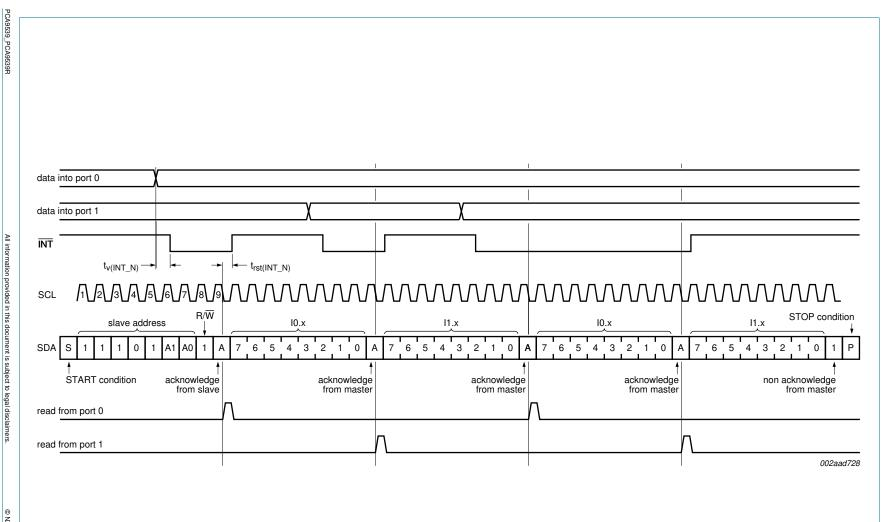
**Remark:** Transfer of data can be stopped at any moment by a STOP condition. When this occurs, data present at the latest acknowledge phase is valid (output mode). It is assumed that the command byte has previously been set to '00' (read input port register).
