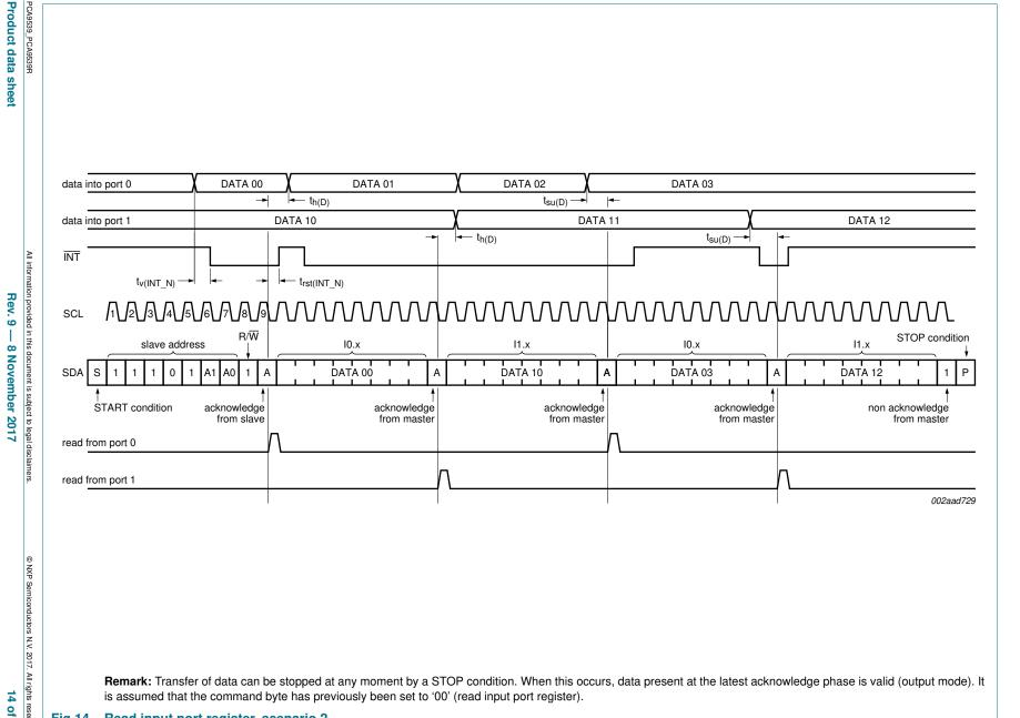
Remark: Transfer of data can be stopped at any moment by a STOP condition. When this occurs, data present at the latest acknowledge phase is valid (output mode). It is assumed that the command byte has previously been set to '00' (read input port register).
