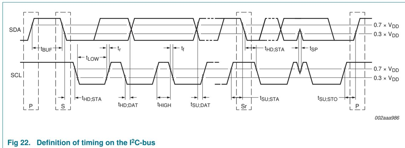
Fig 22. Definition of timing on the I<sup>2</sup>C-bus
