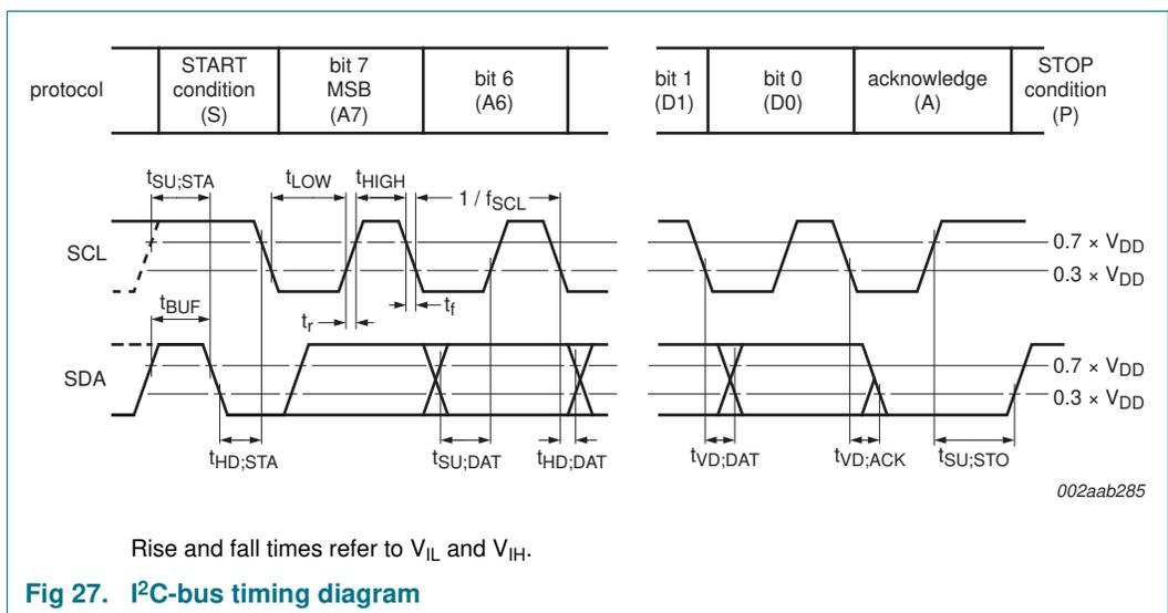
Fig 27. I<sup>2</sup>C-bus timing diagram
