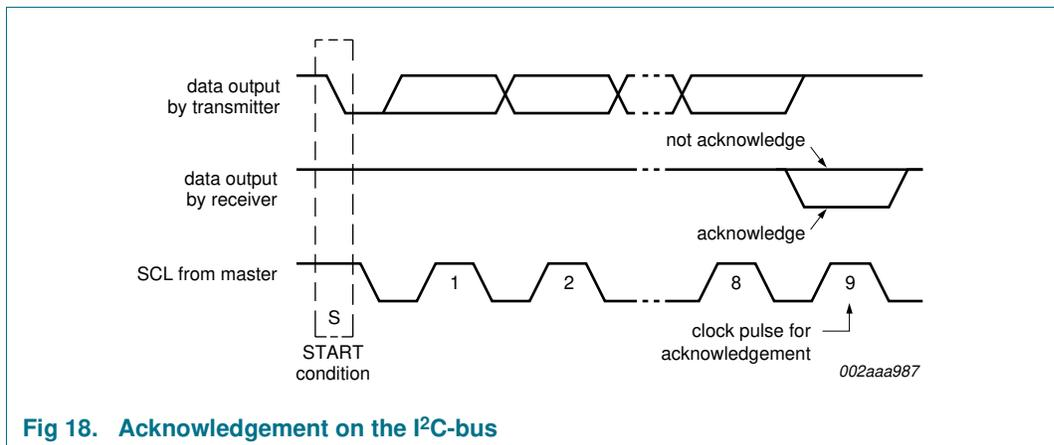
Fig 18. Acknowledgement on the I<sup>2</sup>C-bus
