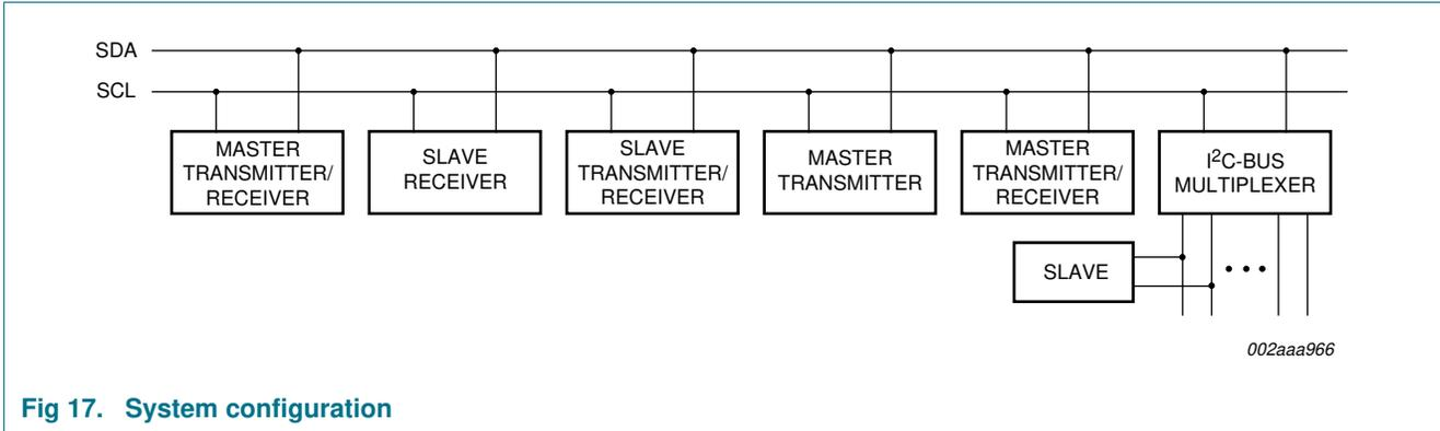
Fig 17. System configuration
