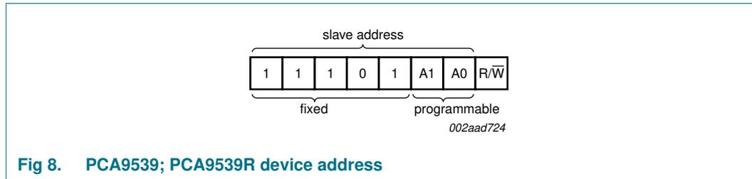
Fig 8. PCA9539; PCA9539R device address
