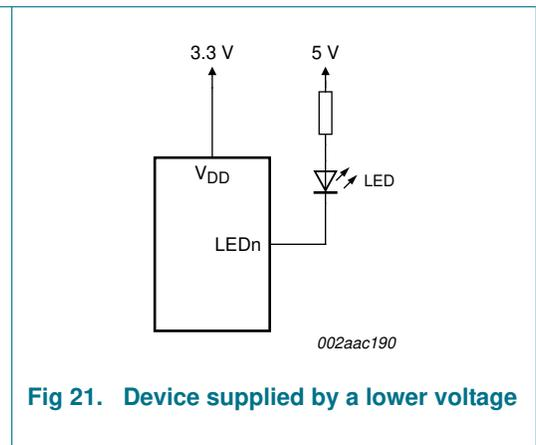
Fig 21. Device supplied by a lower voltage
