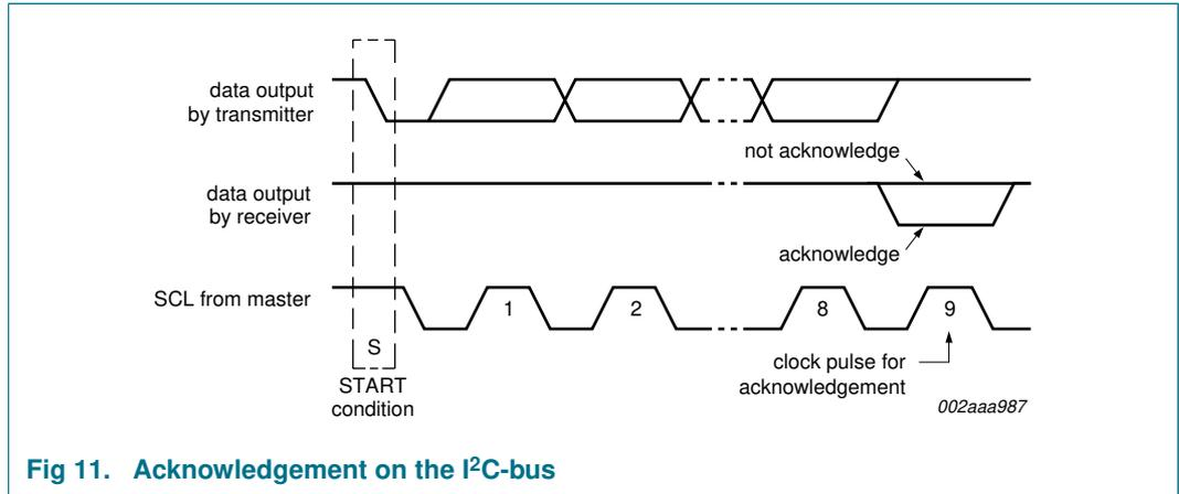
Fig 11. Acknowledgement on the I<sup>2</sup>C-bus
