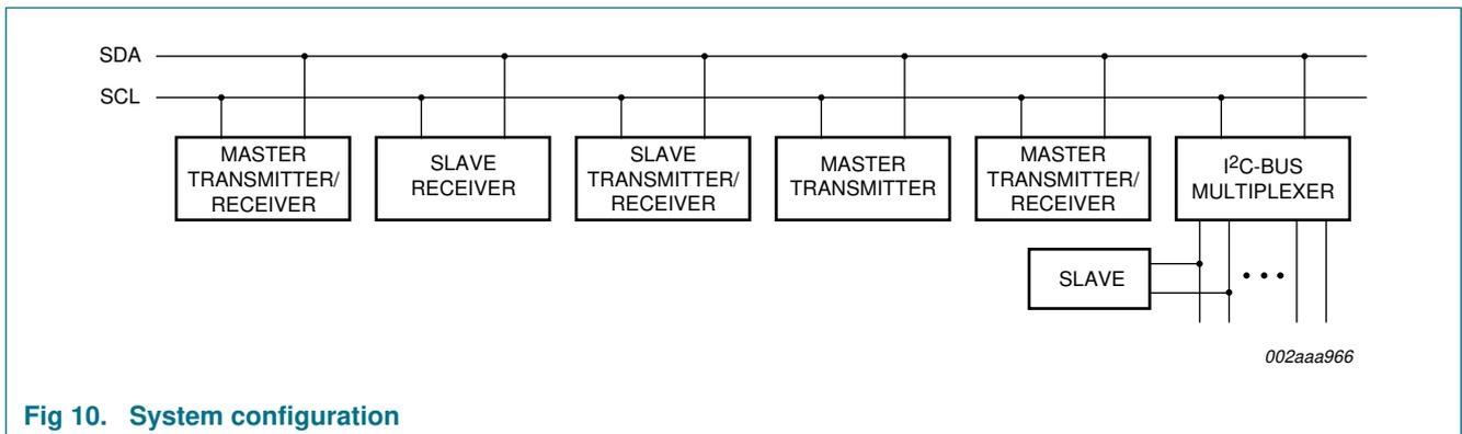
Fig 10. System configuration
