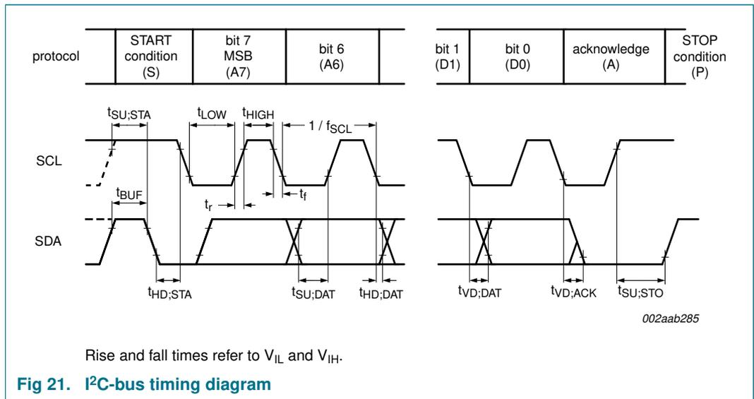
Fig 21. I<sup>2</sup>C-bus timing diagram
