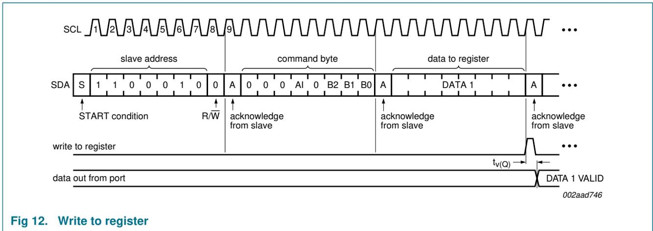
Fig 12. Write to register
