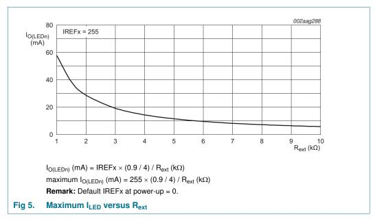
**Example 1:** If  $R_{ext}$  = 1  $k\Omega$ ,  $I_{O}$ \_LED\_MIN = 225  $\mu$ A,  $I_{O}$ \_LED\_MAX = 57.375 mA (as shown in Figure 6).
