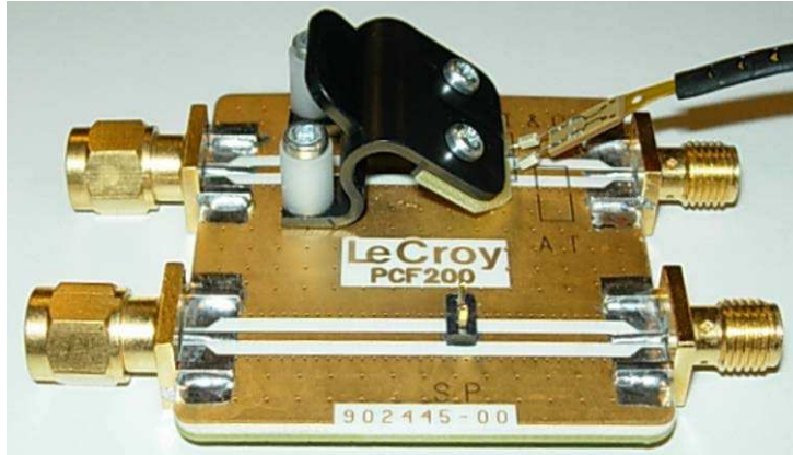
Figure 15. Differential probe properly connected to the fixture (Solder-In configuration)
