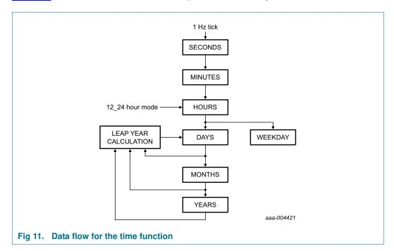
During read/write operations, the time counting circuits (memory locations 04h through 0Ah) are blocked.
