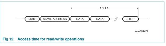
Because of this method, it is very important to make a read or write access in one go, that is, setting or reading seconds through to years should be made in one single access. Failing to comply with this method could result in the time becoming corrupted.
