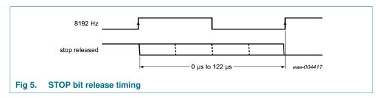
The first increment of the time circuits is between 0.507813 s and 0.507935 s after STOP bit is released. The uncertainty is caused by the prescaler bits  $F_0$  and  $F_1$  not being reset (see Table 7) and the unknown state of the 32 kHz clock.
