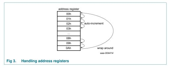
All 11 registers (see <u>Table 5</u>) are designed as addressable 8-bit parallel registers although not all bits are implemented. The first two registers (memory address 00h and 01h) are used as control and status register. The register at address 02h is an offset register allowing the fine-tuning of the clock; and at 03h is a free RAM byte. The addresses 04h through 0Ah are used as counters for the clock function (seconds up to years counters).
