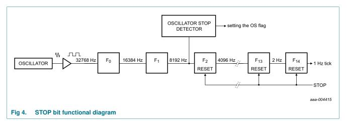
The time circuits can then be set and do not increment until the STOP bit is released (see Figure 5 and Table 7).
