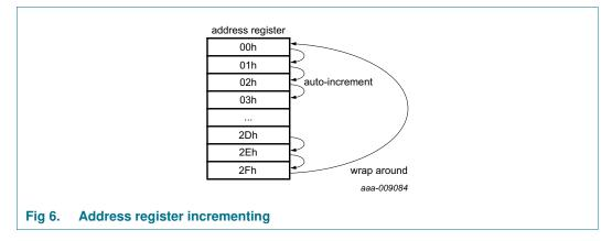
All registers (see Table 5 on page 9, Table 6 on page 11, and Table 7 on page 13) are designed as addressable 8-bit parallel registers although not all bits are implemented. Figure 7 gives an overview of the address map.
