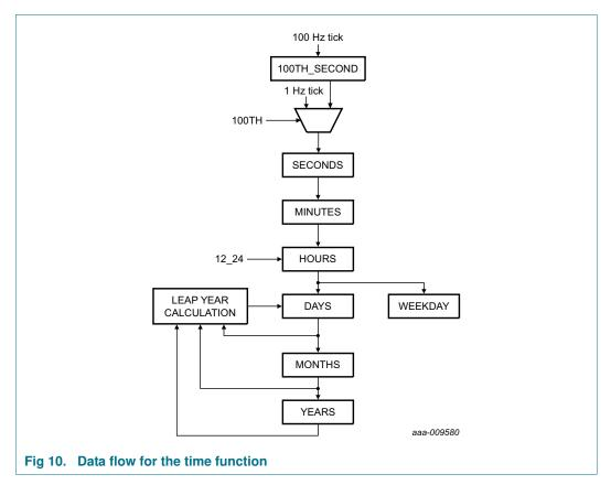
During read operations, the time counting circuits (memory locations 00h through 07h) are copied into an output register. The RTC continues counting in the background.
