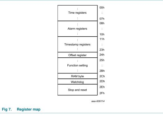
The 100th seconds, seconds, minutes, hours, days, months, and years as well as the corresponding alarm registers are all coded in Binary Coded Decimal (BCD) format. When one of the RTC registers is read, the contents of all time counters are frozen. Therefore, faulty reading of the clock and calendar during a carry condition is prevented.
