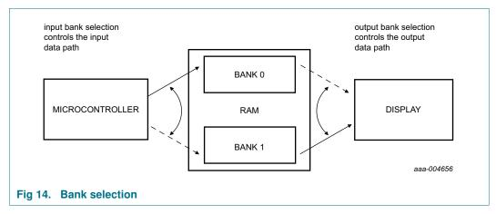
In the static drive mode, the bank-select command may request the contents of row 2 to be selected for display instead of the contents of row 0. In the 1:2 multiplex mode, the contents of rows 2 and 3 may be selected instead of rows 0 and 1. This gives the provision for preparing display information in an alternative bank and to be able to switch to it once it is assembled.
