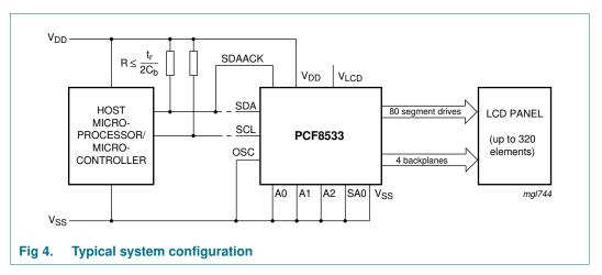
The host microcontroller maintains the 2-line  $I^2C$ -bus communication channel with the PCF8533. The internal oscillator is enabled by connecting pin OSC to pin  $V_{SS}$ . The appropriate biasing voltages for the multiplexed LCD waveforms are generated internally. The only other connections required to complete the system are the power supplies ( $V_{DD}$ ,  $V_{SS}$ , and  $V_{LCD}$ ) and the LCD panel chosen for the application.
