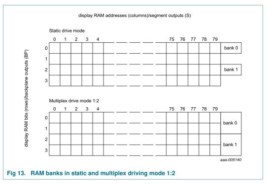
There are two banks; bank 0 and bank 1. <u>Figure 13</u> shows the location of these banks relative to the RAM map. Input and output banks can be set independently from one another with the Bank-select command (see <u>Table 9 on page 6</u>). <u>Figure 14</u> shows the concept.
