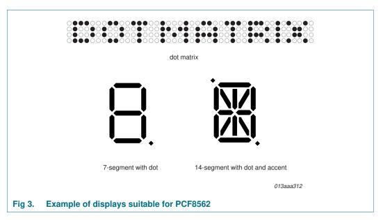
The possible display configurations of the PCF8562 depend on the number of active backplane outputs required. A selection of display configurations is shown in <u>Table 4</u>. All of these configurations can be implemented in the typical system shown in <u>Figure 4</u>.
