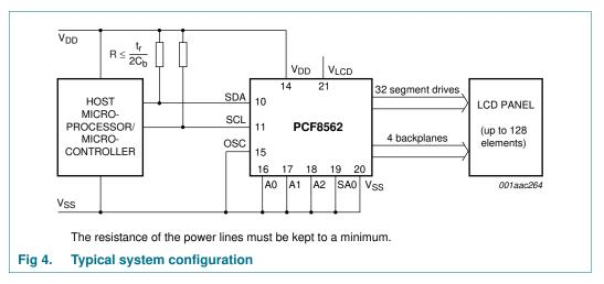
The host microcontroller maintains the 2-line  $I^2C$ -bus communication channel with the PCF8562. The internal oscillator is enabled by connecting pin OSC to pin  $V_{SS}$ . The appropriate biasing voltages for the multiplexed LCD waveforms are generated internally. The only other connections required to complete the system are to the power supplies  $(V_{DD}, V_{SS}, \text{ and } V_{LCD})$  and the LCD panel chosen for the application.
