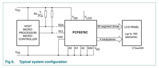
The host microprocessor or microcontroller maintains the 2-line I<sup>2</sup>C-bus communication channel with the PCF8576C.
