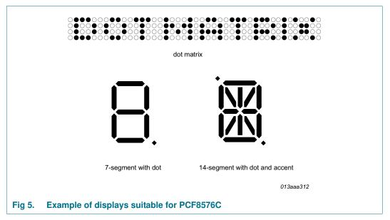
The possible display configurations of the PCF8576C depend on the number of active backplane outputs required. A selection of display configurations is shown in <u>Table 5</u>. All of these configurations can be implemented in the typical system shown in Figure 6.
