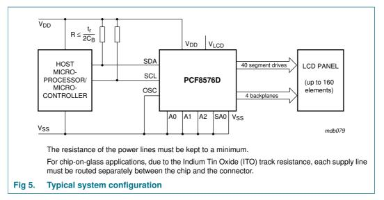
The host microprocessor or microcontroller maintains the 2-line  $I^2C$ -bus communication channel with the PCF8576D. The internal oscillator is enabled by connecting pin OSC to pin  $V_{SS}$ . The appropriate biasing voltages for the multiplexed LCD waveforms are generated internally. The only other connections required to complete the system are to the power supplies ( $V_{DD}$ ,  $V_{SS}$  and  $V_{LCD}$ ) and the LCD panel chosen for the application.
