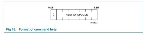
After the last command byte, one or more display data bytes may follow. Display data bytes are stored in the display RAM at the address specified by the data pointer and the subaddress counter. Both data pointer and subaddress counter are automatically updated and the data directed to the intended PCF8576D device.
