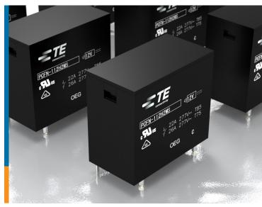
TE Connectivity has expanded the PCFN Solar Relay line to include a new high performance relay with larger ( > 1.8 mm) contact gaps to support extended insulation requirements for use in photovoltaic applications. With the same mechanical dimensions as the standard PCFN solar relays, the new high performance version has increased thermal performance up to 90°C and features a 1.5 W coil with low holding power of 200 mW to help lower energy costs.
