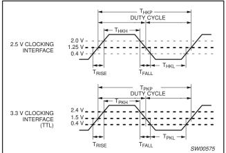
Figure 7. 2.5 V/3.3 V clock waveforms
