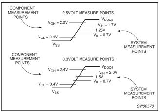
Figure 2. 3.3 V clock waveforms
