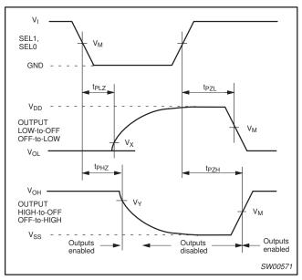
Figure 3. State enable and disable times
