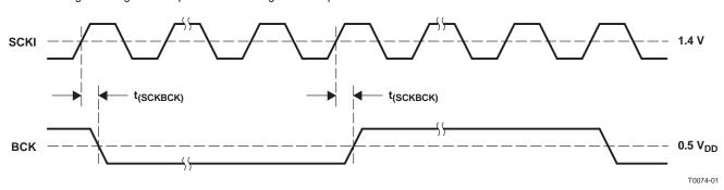
Figure 22. Audio Clock Interface Timing (Master Mode: BCK Works as Output)
