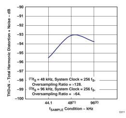
Figure 25. Total Harmonic Distortion + Noise vs f<sub>SAMPLE</sub> Condition
