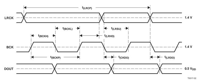
Figure 20. Audio Data Interface Timing (Slave Mode: LRCK and BCK Work as Inputs)
