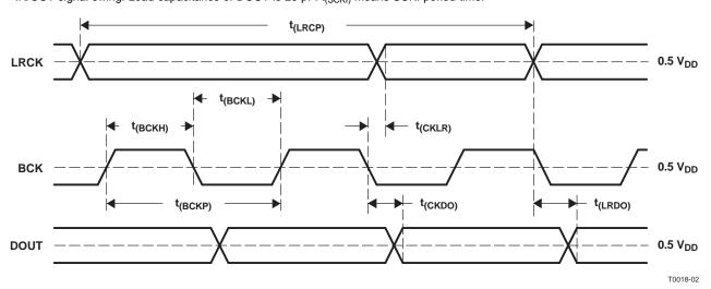
Figure 21. Audio Data Interface Timing (Master Mode: LRCK and BCK Work as Outputs)
