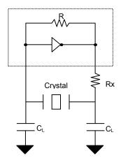
$$\begin{split} C_\text{L} &= 2^*(C_P - C_S), \\ \text{Where } C_P &= \text{Load capacitance of crystal} \\ C_S &= \text{Stray capacitance due to } C_\text{IN, } \text{PCB, } \text{Trace etc.} \end{split}$$
