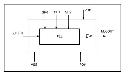
Figure 1. Block Diagram
