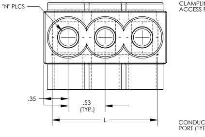
THREE PORT CONNECTOR BLOCK SHOWN WITH PLASTIC CLOSURE PLUGS REMOVED.
