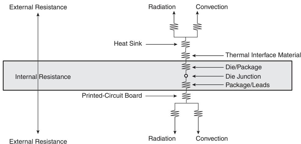
Note the internal versus external package resistance.
