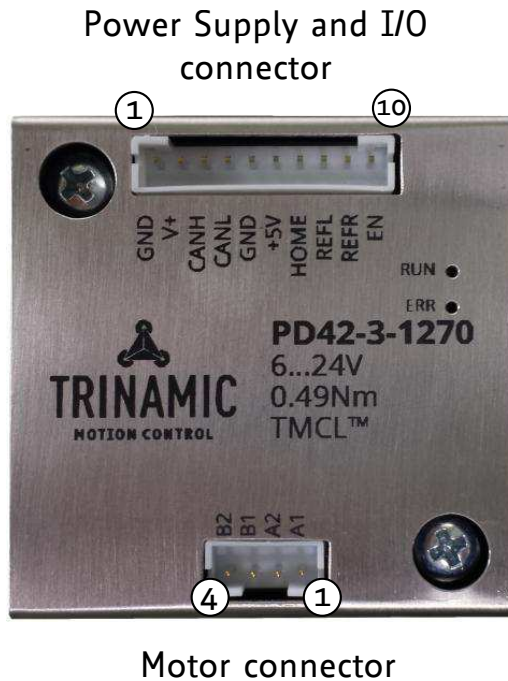
Figure 11: PD42-1270 connectors
