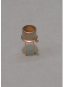
PACKAGE DIMENSIONS INCH [mm] 45 0.50 [12.7] MIN 0.040 0.145 [3.68] 0.145 [3.68] Ø0.019 [0.48] Ø0.016 [0.41] WIRE BOND Ø0.195 [4.95] Ø0.178 [4.52] 0.100 [2.54] ANODE CATHODE & CASE PHOTODIODE CHIP WINDOW CAP Ø0.209 5.31 0.025 [0.64] (WELDED) 0.027 [0.69] 0.022 0.56 HEADER SOUARE Ø0.012 [Ø0.30] TO-46 HERMETIC CAN PACKAGE ACTIVE AREA ACTIVE AREA =  $0.073 \text{ mm}^2$
