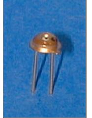
High-Speed GaAIAs Infrared Point Source Emitter Peak Wavelength 850 nm, Type PDI-E824
