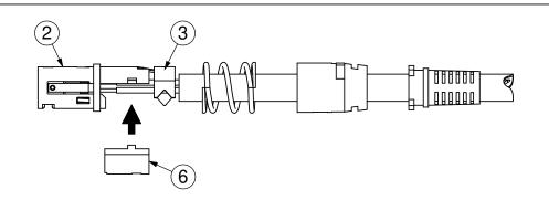
STEP 4 crimp the clamp (3) onto wires, assemble metal cover (6) onto metal sleeve (2)
