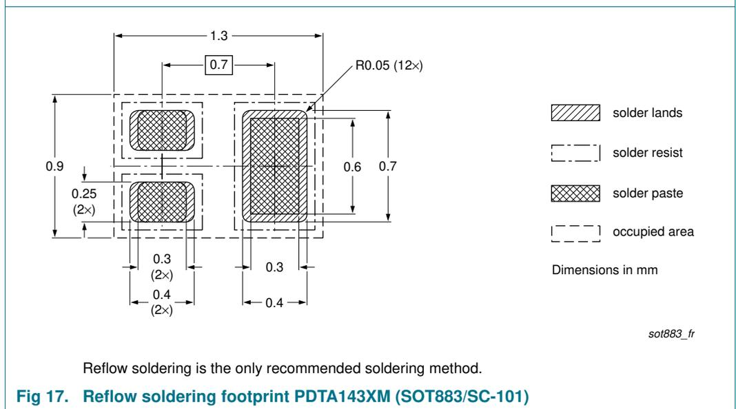
**Fig 17. Reflow soldering footprint PDTA143XM (SOT883/SC-101)**
