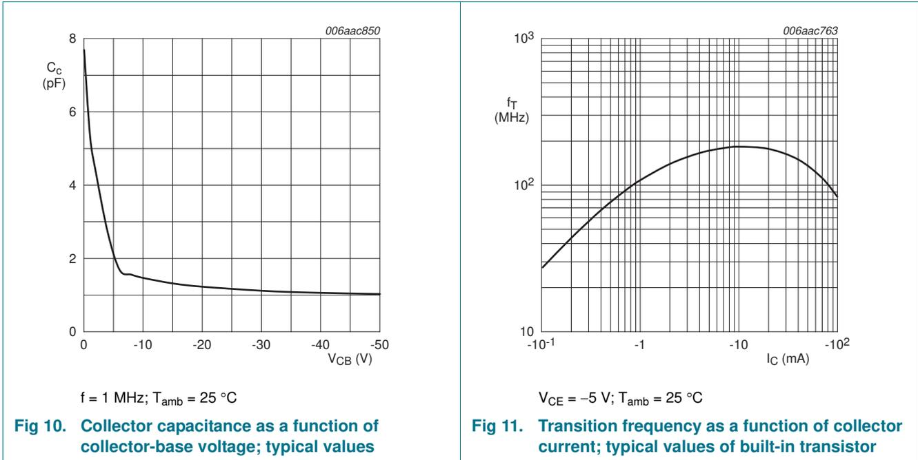
**Fig 10. Collector capacitance as a function of collector-base voltage; typical values**
