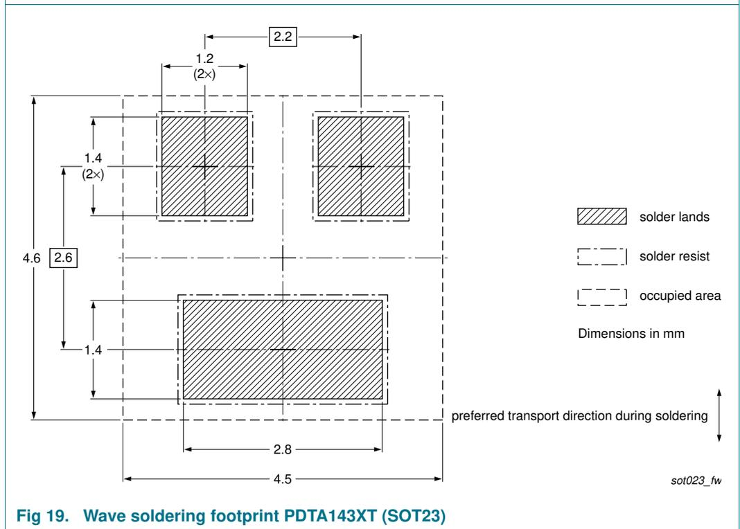
**Fig 19. Wave soldering footprint PDTA143XT (SOT23)**
