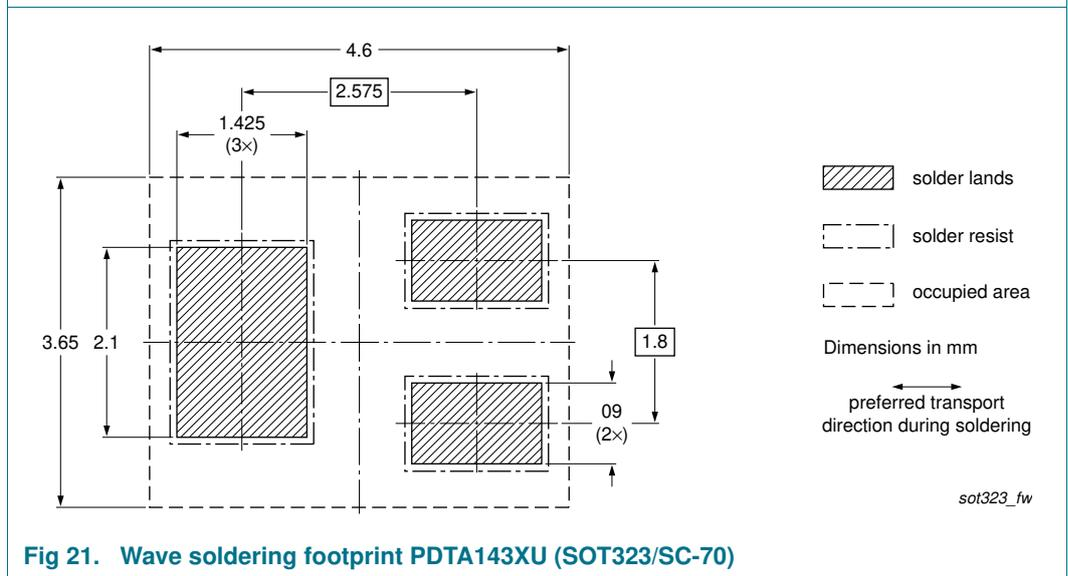
**Fig 21. Wave soldering footprint PDTA143XU (SOT323/SC-70)**
