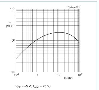
Fig 11. Transition frequency as a function of collector current; typical values of built-in transistor
