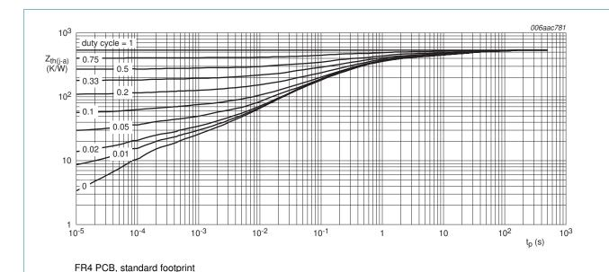
Fig 2. Transient thermal impedance from junction to ambient as a function of pulse duration for PDTA143XE (SOT416); typical values
