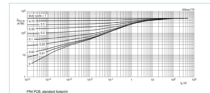
Fig 4. Transient thermal impedance from junction to ambient as a function of pulse duration for PDTA143XT (SOT23); typical values
