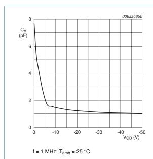
Fig 10. Collector capacitance as a function of collector-base voltage; typical values
