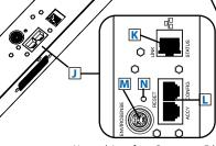
Network Interface: Connect to Ethernet for remote monitoring via SNMP, Web or Telnet. Add optional ENVIROSENSE accessory for temperature/humidity monitoring and dry contact interface.
