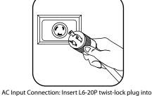
compatible L6-20R utility, generator or UPS outlet. For international applications, connect user-supplied power cord with region-specific plug to C20 power inlet.
