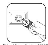
AC Input Connection: Insert L5-30P twist-lock plug into compatible L5-30R utility, generator or UPS outlet.
