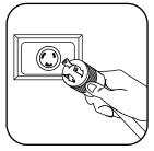
AC Input Connection: Insert L5-20P twist-lock plug into compatible L5-20R utility, generator or UPS outlet. (Included adapter converts L5-20P to 5-20P.)
