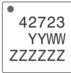
Figure 19 • Package Marking Specifications for PE42723
