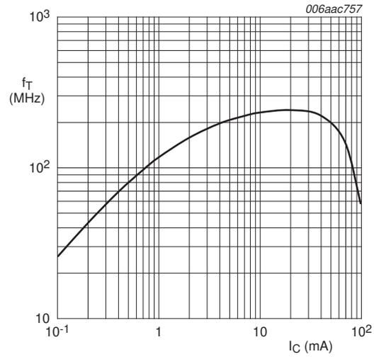
$V_{\text{CE}} = 5 \text{ V}; T_{\text{amb}} = 25 \text{ }^\circ\text{C}$
