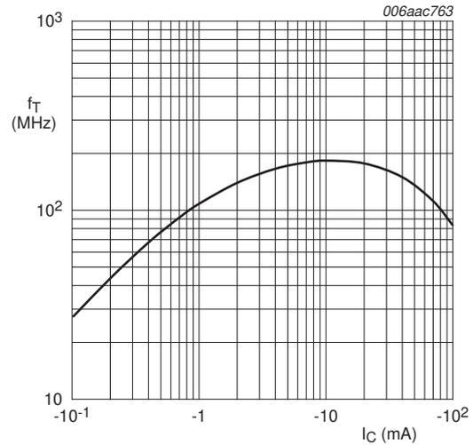
$V_{CE} = -5 \text{ V}; T_{amb} = 25 \text{ }^\circ\text{C}$
