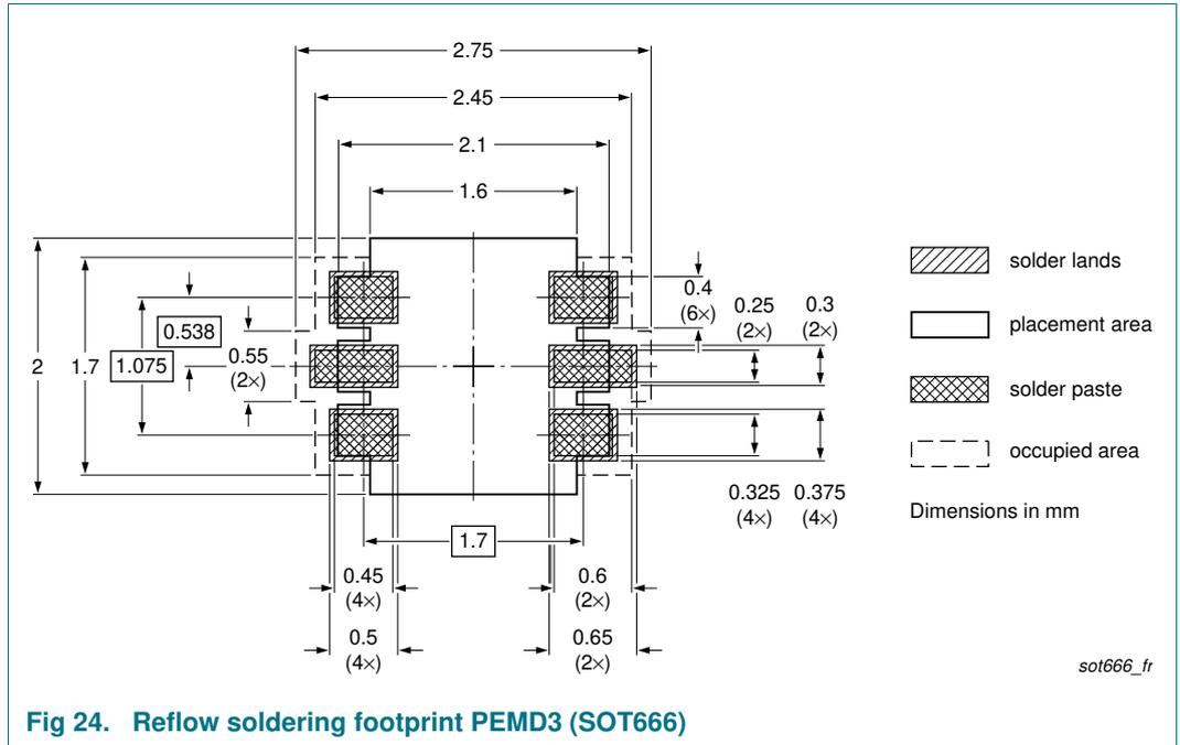
Fig 24. Reflow soldering footprint PEMD3 (SOT666)
