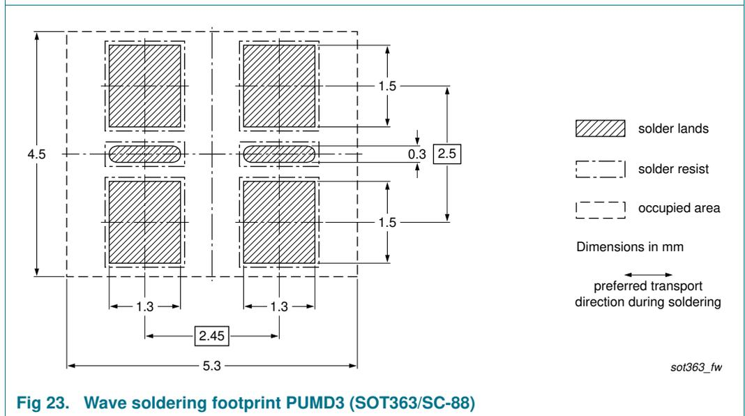
**Fig 23. Wave soldering footprint PUMD3 (SOT363/SC-88)**
