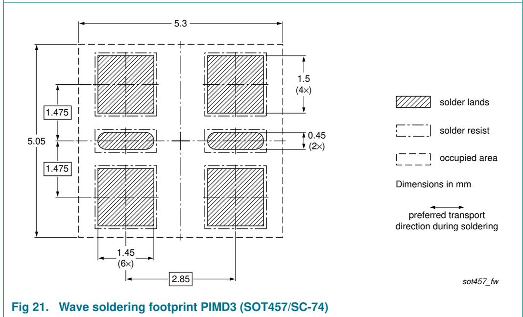
Fig 21. Wave soldering footprint PIMD3 (SOT457/SC-74)
