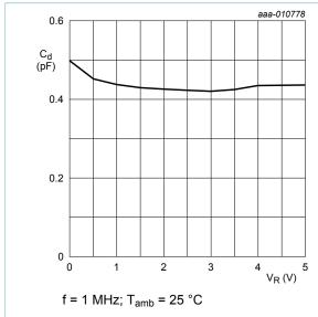
Diode capacitance as a function of reverse Fig. 3. voltage; typical values
