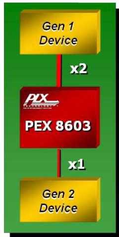
Figure 5. Gen 1 to Gen 2 Bandwidth Bridge
