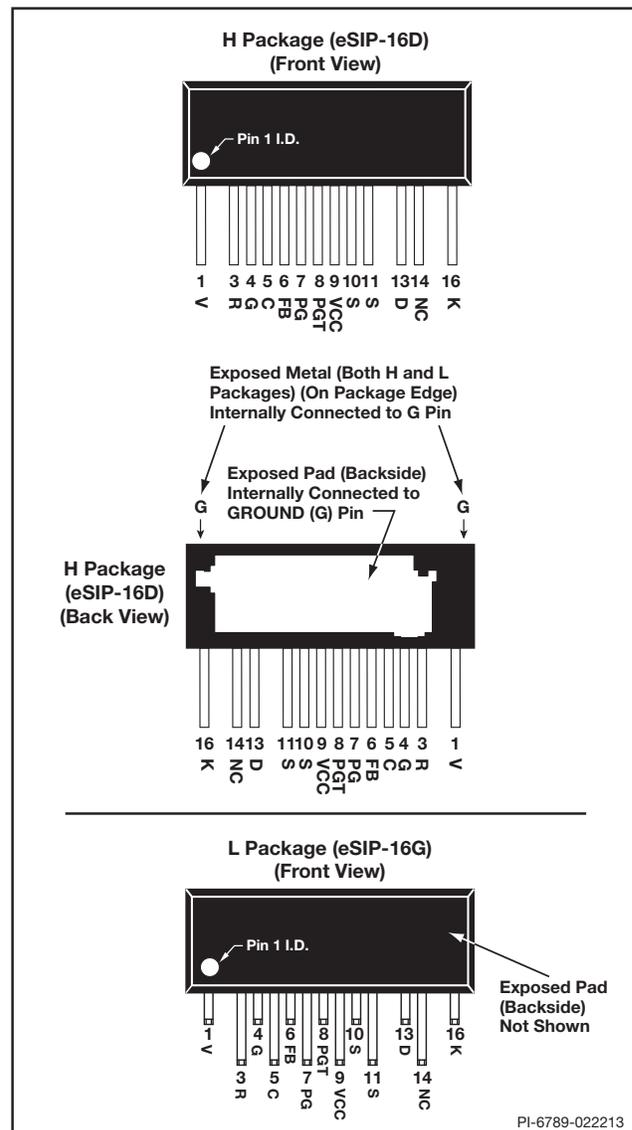
Figure 2. Pin Configuration.
