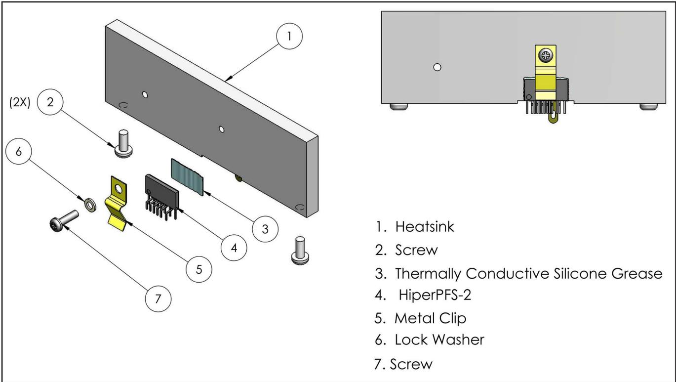
Figure 17. Heat Sink Assembly – with Metal Clip.
