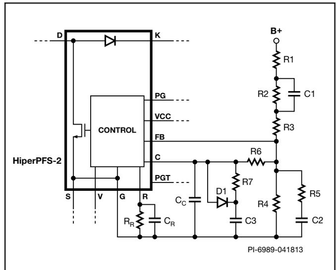
Figure 15. Recommended Feedback Circuit.
