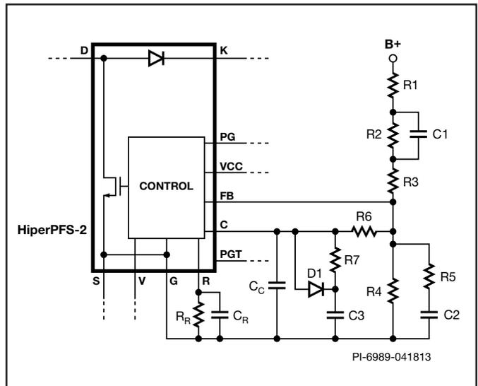
Figure 15. Recommended Feedback Circuit.
