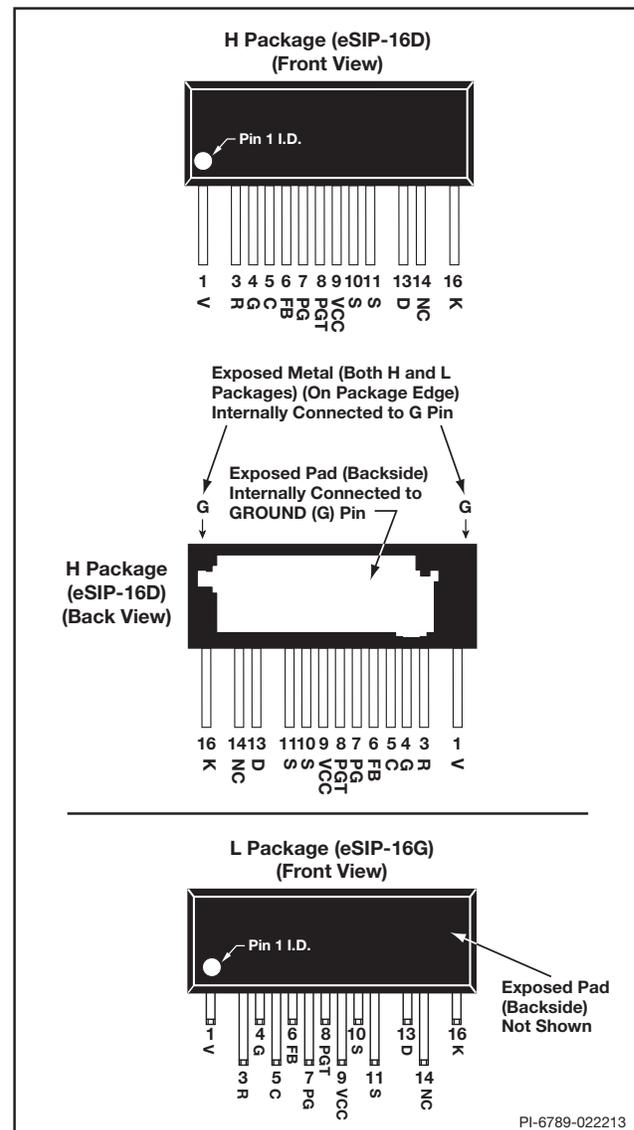
Figure 2. Pin Configuration.
